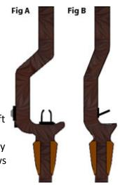
A basic moulded riser (Figure B) does not have this feature. If you have an 80's or early 90's vintage bow, you almost certainly have this type of riser. In a non-cutaway bow, the actual centre-shot of the bow is very close to (if not right against) the edge of the riser. This type of riser typically uses a flipper/plunger style rest mounted right against the side of the bow, where a cutaway riser generally cannot.
